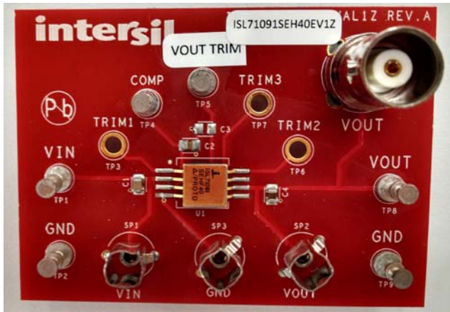
FIGURE 6. VOLTAGE REFERENCE EVALUATION BOARD (FRONT)
